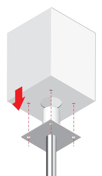
2) Once the shade is resting on the mounting plate and correctly oriented, affix it by passing the supplied 1/4-20 x 11/2" screws up through the holes in the mounting plate and into the bottom of the shade. Then inside the shade, place washers over and then turn a nut onto that screw. Tighten all four screws into their nuts so the shade is securely held in place, but do not over-tighten to avoid damage to the shade.
