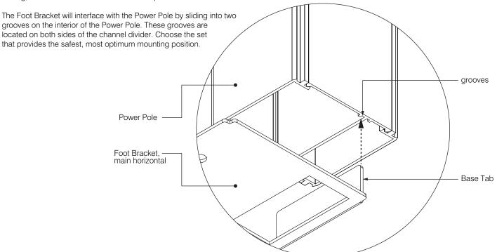
Step 1 Insert Base Tab into Power Pole grooves
