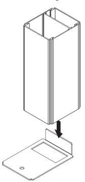
Step 2 Locate and drill hole into mounting surface
