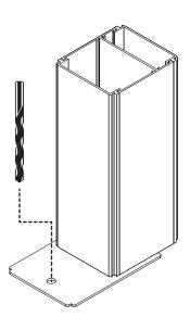
Step 3 Secure fastener through hole in Foot Bracket into mounting surface
